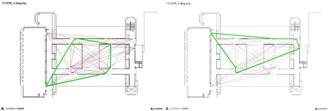
Fig. 5. Closed loop path for 2 vehicles by solving graph partitioning problem. Left: TSP path for Vehicle 1; right: TSP path for Vehicle 2.
