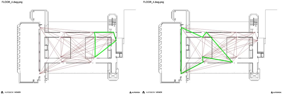
Fig. 3. Closed loop path for 2 vehicles using spectral clustering. Left: TSP path for Vehicle 1; right: TSP path for Vehicle 2.
