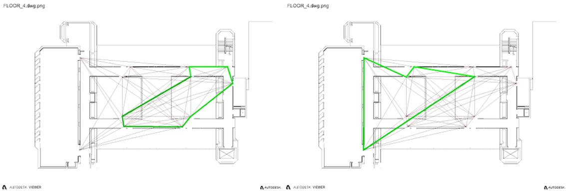
Fig. 4. Closed loop path for 2 vehicles by solving CVRP. Left: CVRP path for Vehicle 1; right: CVRP path for Vehicle 2.
